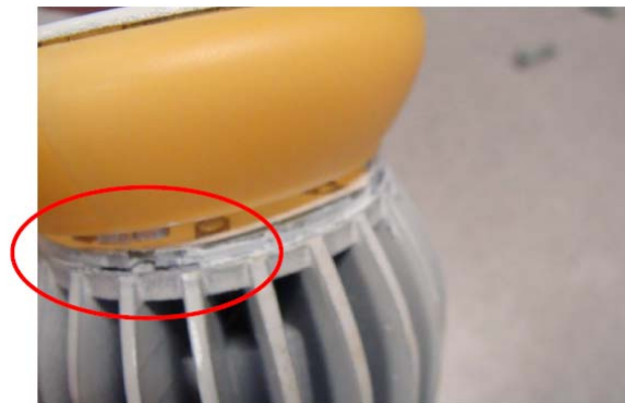
Figure 10 Bottom tabs on remote phosphor engage bottom slot in heat sink
